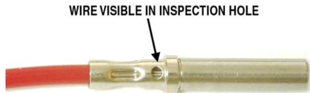
Figure 3 – Correctly Crimped Terminal
