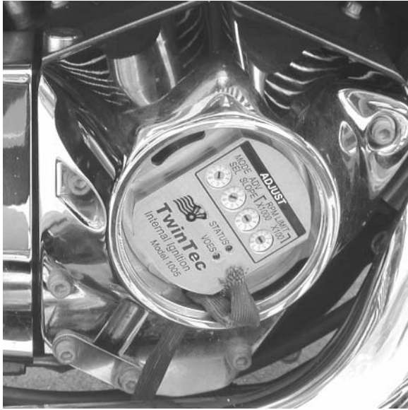
Figure 2 - Installing Unit (Note Orientation)
