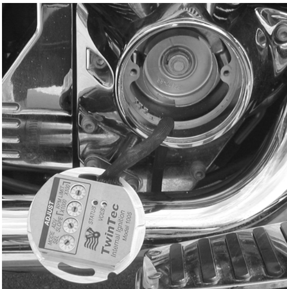
Figure 1 - Feeding Harness Thru Exit Hole
