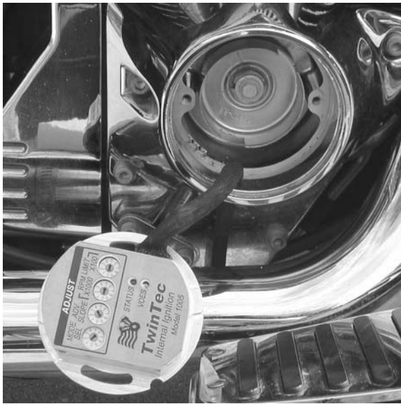
Figure 1 - Feeding Harness Thru Exit Hole
