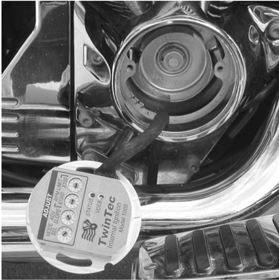
3. You can completely remove the Gill ignition module and associated wiring, except for the White/Black switched +12 volt wire at the coils and the White/Violet tach wire.
