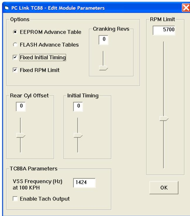
Regardless of the advance table selection, you can also select the Fixed Initial Timing and/or Fixed RPM Limit options. If you select one of these options, the corresponding slider control appears and allows you to enter a value. Fixed initial timing and RPM limit override any module switch settings. These options are primarily intended for engine builders and tuners.
