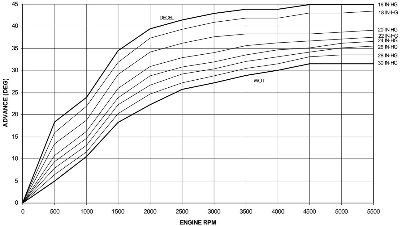
Figure 5 - Graph Representing Advance Slope Setting 9 (Most Aggressive)
