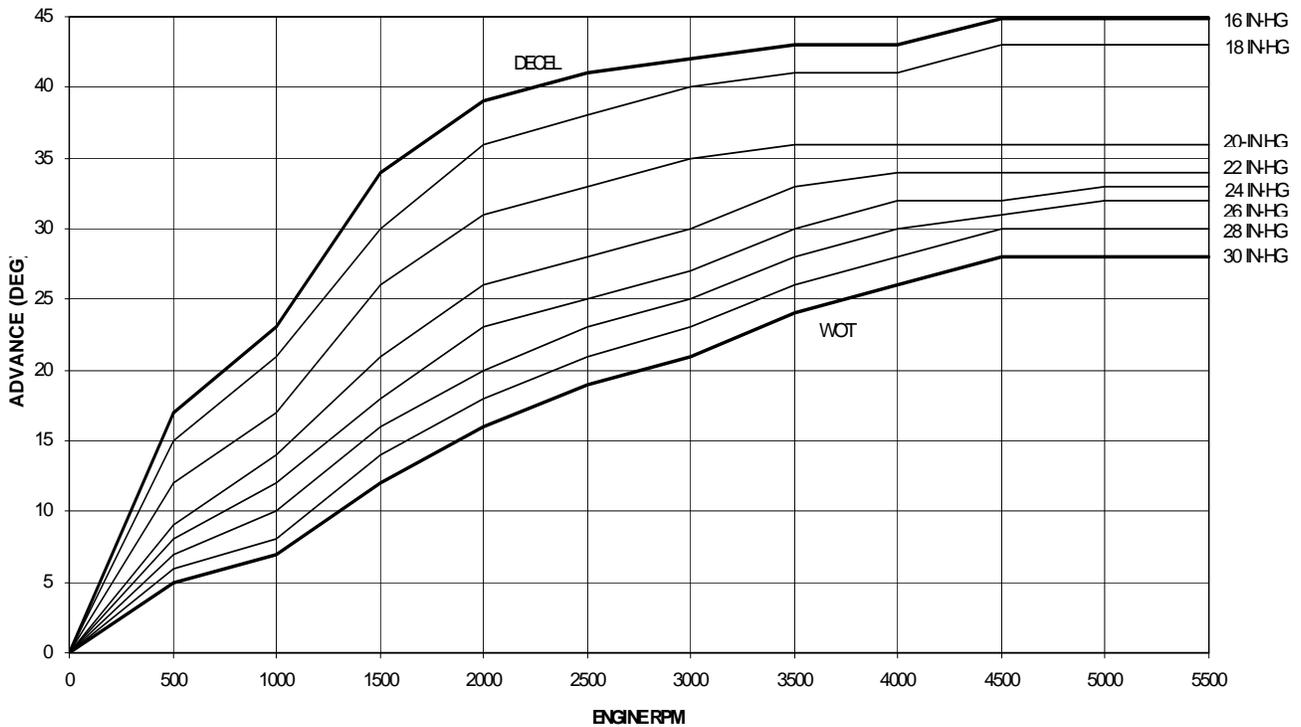
Figure 4 - Graph Representing Advance Slope Setting 5 (Nominal)
