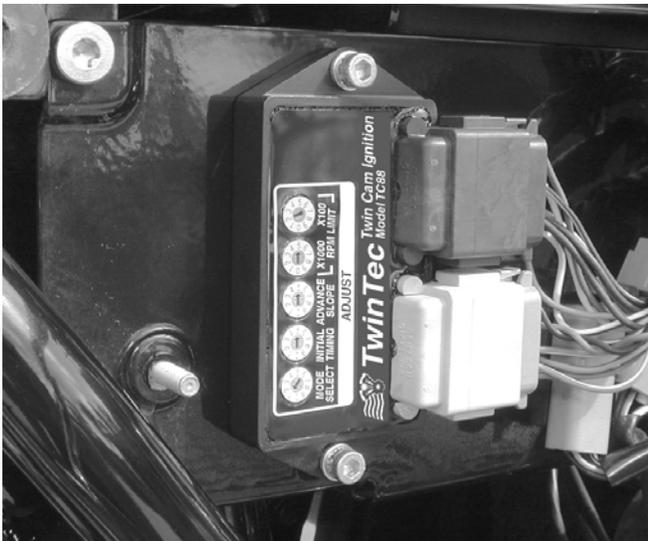
3. Install the new Twin Tec module. Figure 1 shows a typical installation under a side cover. You can reuse the original mounting hardware.
