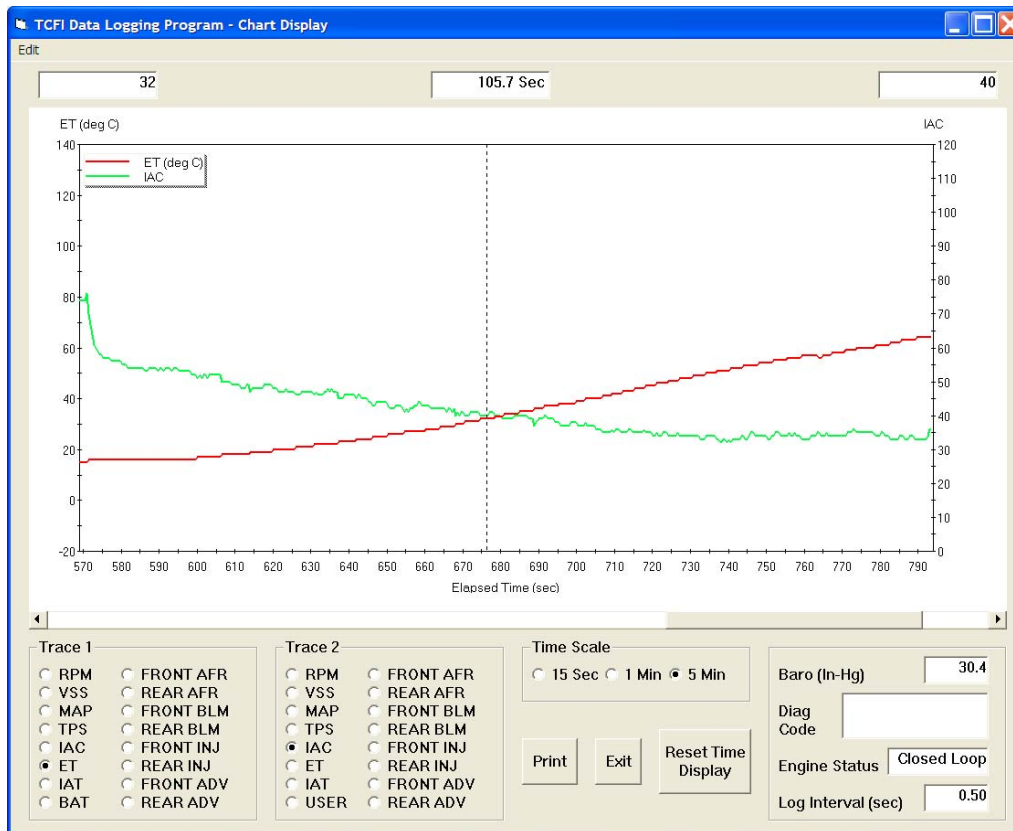
Figure 3 – Cold Start Test Showing ET and IAC Data
