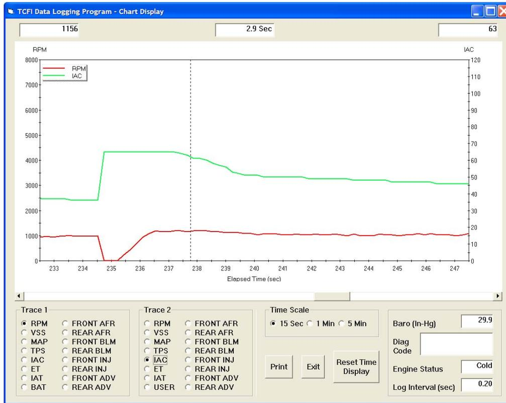
Figure 4 shows data logged from a hot start test using reasonable ET Based IAC Start Adder values (taken from Table 3). Time display has been reset to zero at engine start. RPM and IAC values are displayed. Engine RPM increases smoothly after cranking and then quickly levels off to 1,000 RPM. The correct amount of additional air is being provided during engine start. You can see that the IAC values follow a curve similar to Figure 2.
