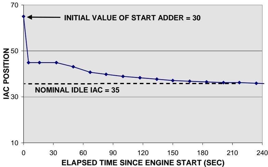
Note: for the example shown in Figure 2, the ET based IAC term is assumed to be zero (engine at 96 deg C). The closed loop correction term is also assumed to be zero.
