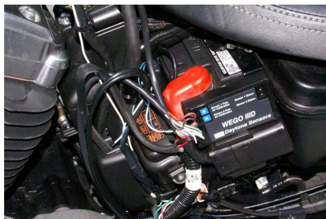
Figure 21 - Typical Sportster® Installation with WEGO IIID Mounted to Side of Battery
