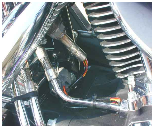
Figure 22 – Typical Sensor Installation
