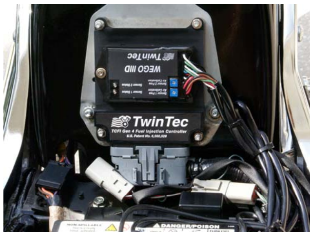
Figure 20 - Typical Twin-Cam Installation with WEGO IIID Mounted on Top of TCFI Unit
