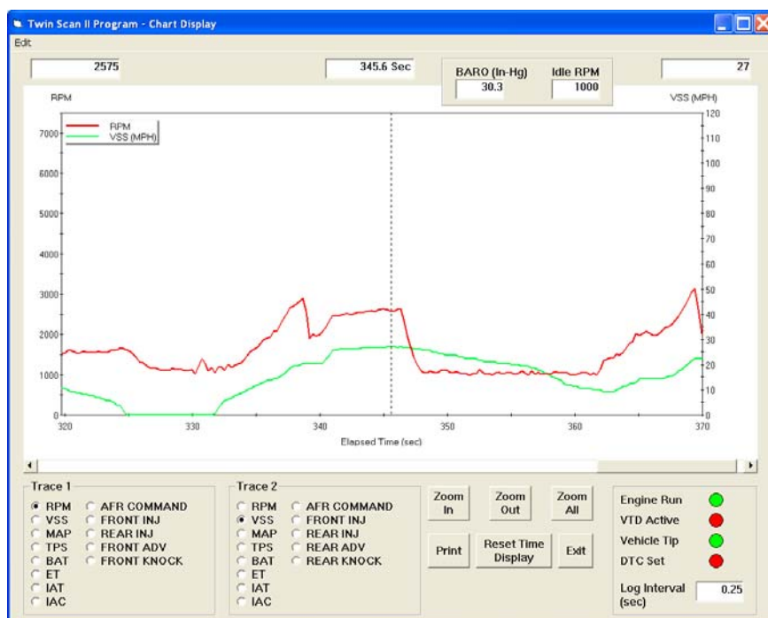
Figure 9 – Data Logging Chart Display
