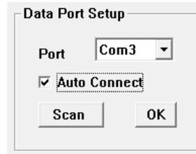
You can test communications between the Twin Scan 4 and the laptop PC by using the Read Firmware ID command on the Help menu (a connection to the motorcycle is not required for this test). If you get an error message, please refer to the Communications Troubleshooting Flowchart on page 21.
