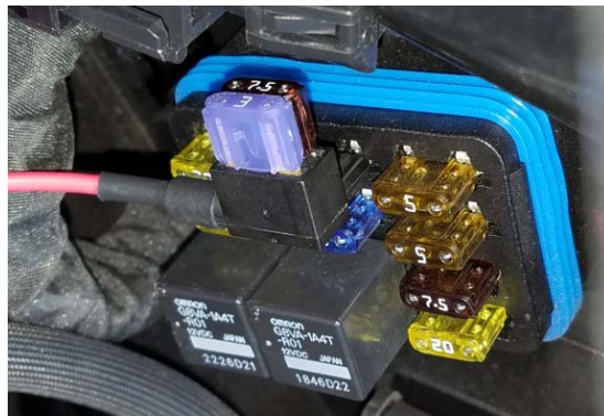
Figure 19C – SYSTEM 7.5A Fuse tap connection for switched uninterrupted power on 2018
