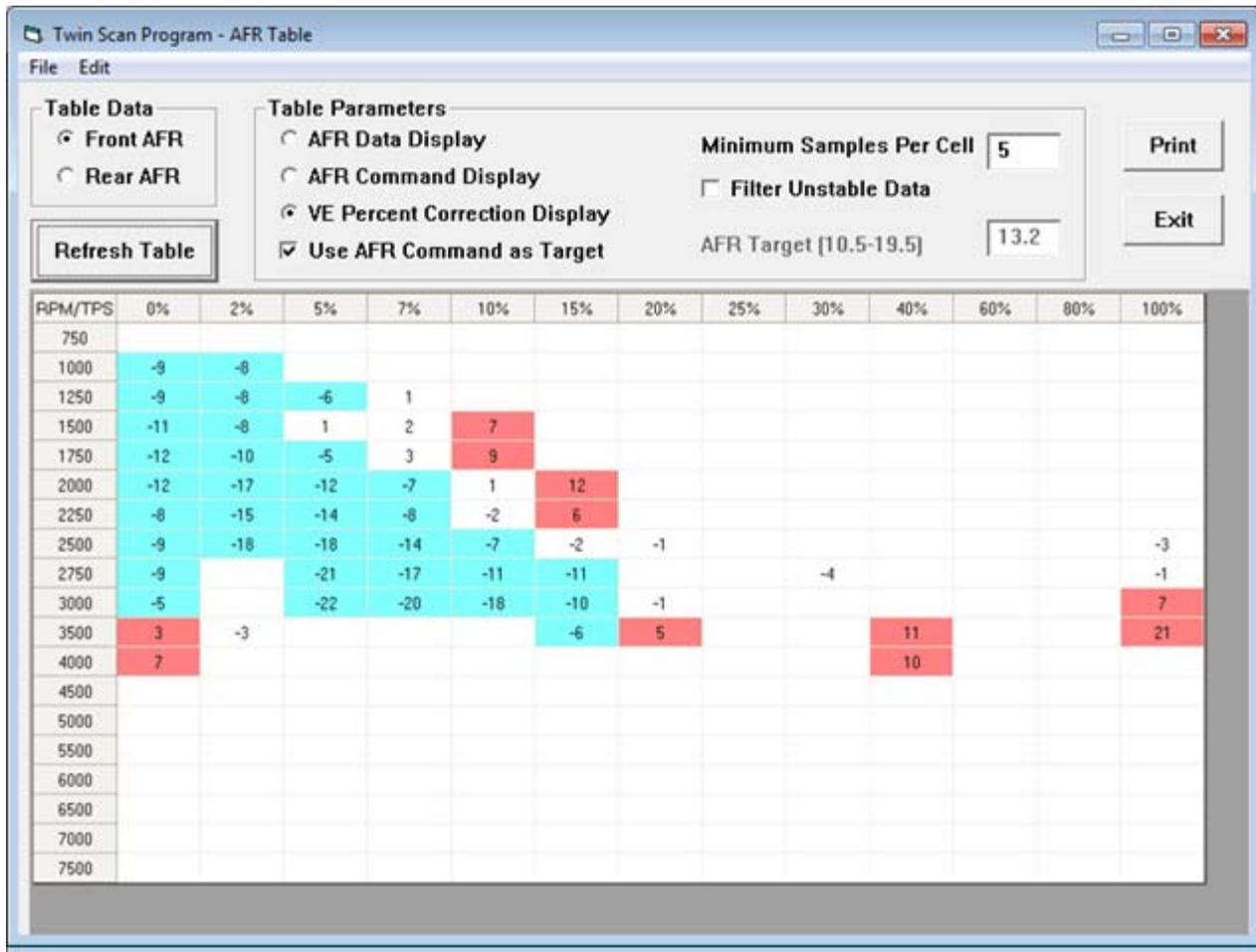
**Target AFR** –manual target AFR value used to determine required percent VE correction. You might use a manual target AFR of 13.2 if you are using the tuning approach outlined in the earlier SEST manual where all SEST AFR table cells are set to 13.2 during tuning.
