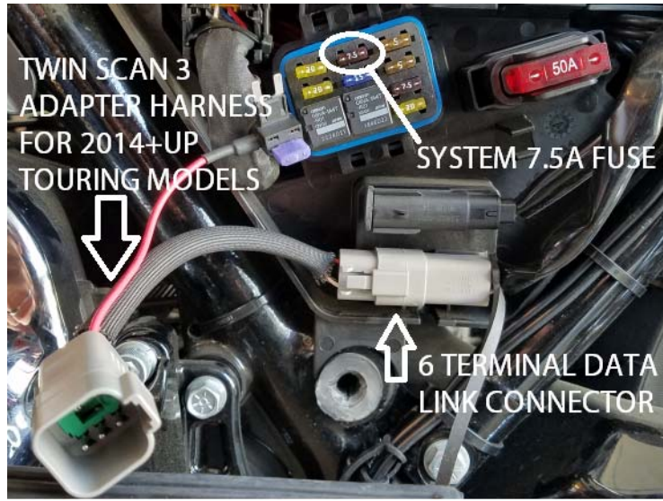
Figure 19B – SYSTEM 7.5A Fuse tap connection for switched uninterrupted power on 2014-2017
