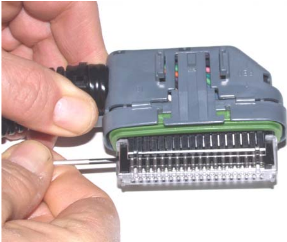
Figure 3 – ECM Connector Disassembly
