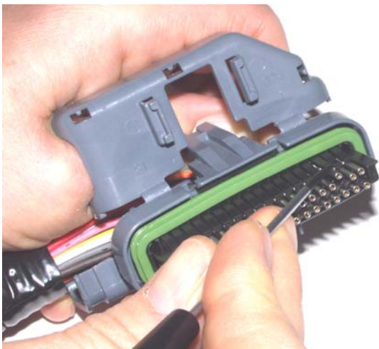
Figure 4 – ECM Connector Terminal Removal
