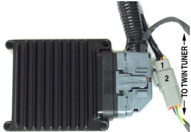
Figure 5 – Completed Wiring at ECM
