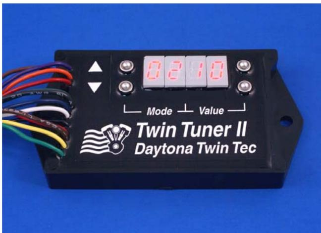
You can use the up/down pushbutton switches to select the mode and change fuel trim and ignition retard values in the RPM and throttle position ranges required by most applications.
