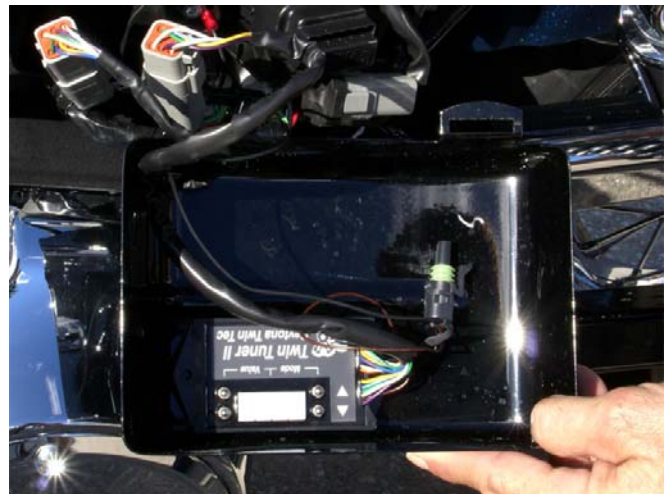
Figure 4 – Typical Dyna® Installation (Twin Tuner II Shown – Twin Tuner Similar)
