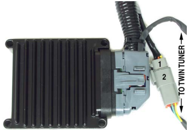
Figure 5 – Completed Wiring at ECM
