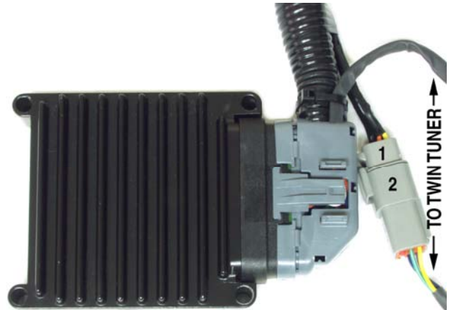
Figure 5 – Completed Wiring at ECM
