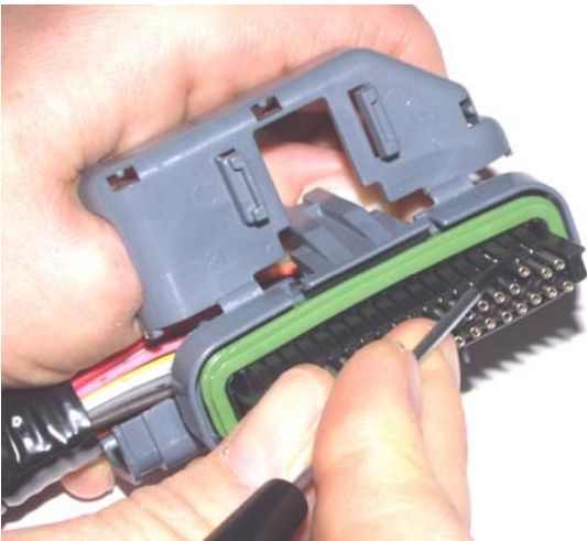
Figure 4 – ECM Connector Terminal Removal
