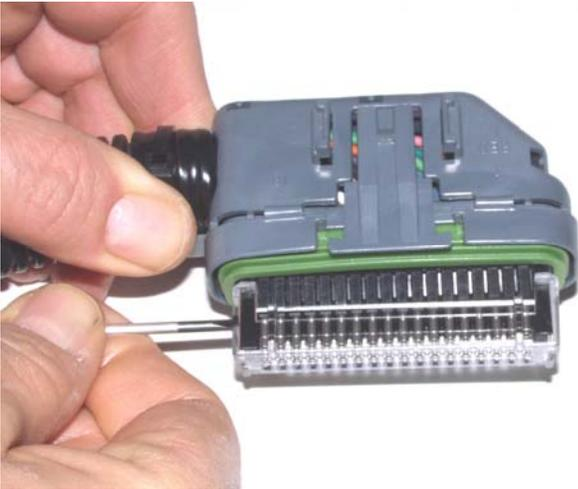
Figure 3 – ECM Connector Disassembly
