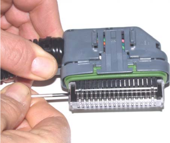
Figure 3 – ECM Connector Disassembly
