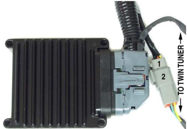
7. Terminal numbers are marked on the back side of the ECM connector. Original equipment wire color codes may vary. Note the color of each wire that you remove. We suggest that you mark up Table 1 with any corrections for future reference.
