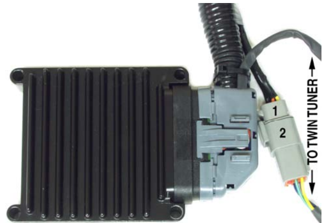
Figure 5 – Completed Wiring at ECM
