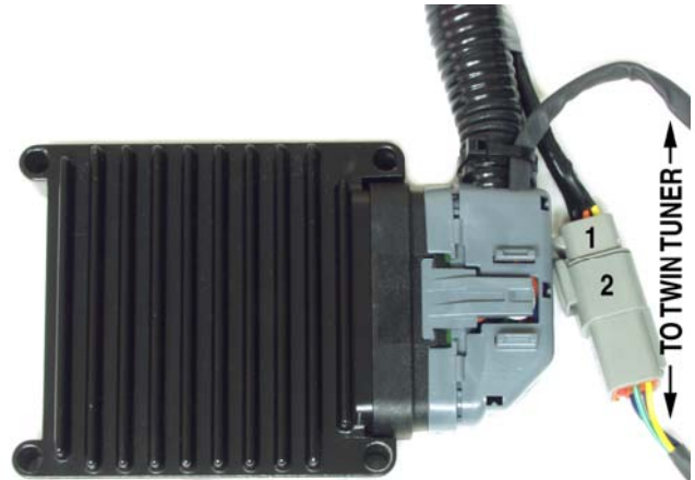
Figure 5 – Completed Wiring at ECM
