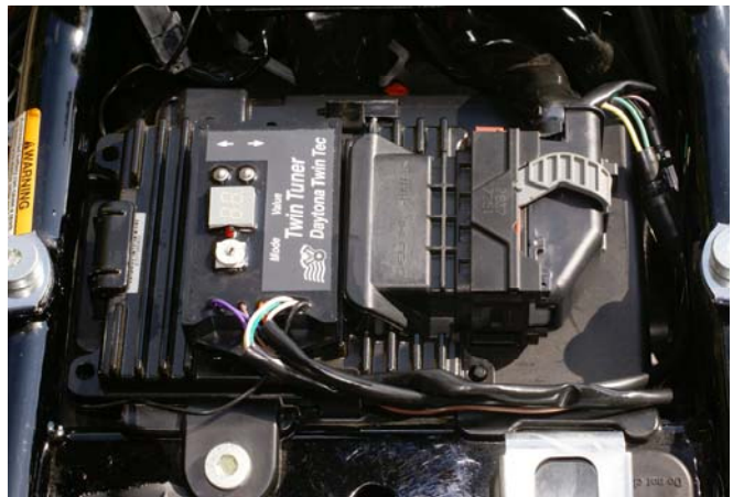
Figure 8 – Completed Twin Tuner Installation
