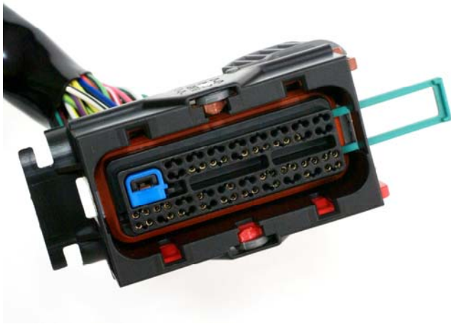
Figure 2 – ECM Connector Retainer Removal
