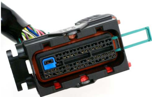
Figure 2 – ECM Connector Retainer Removal
