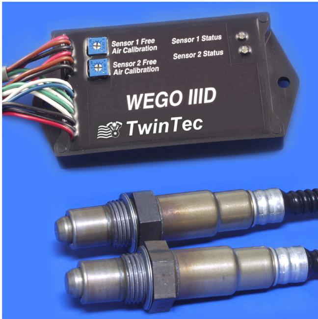
The WEGO includes internal diagnostics for abnormal battery voltage (less than 11 volts or greater than 16.5 volts), sensor open circuit, and sensor short circuit conditions. A fault condition causes the status LEDs to blink at the slow rate.
