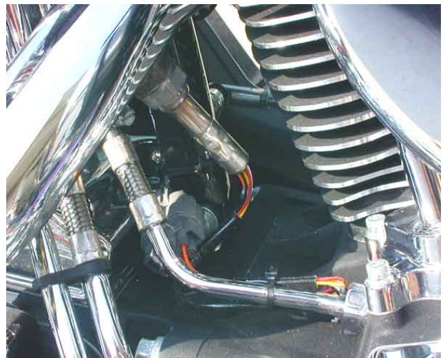
Figure 1 – Typical Sensor Installation
