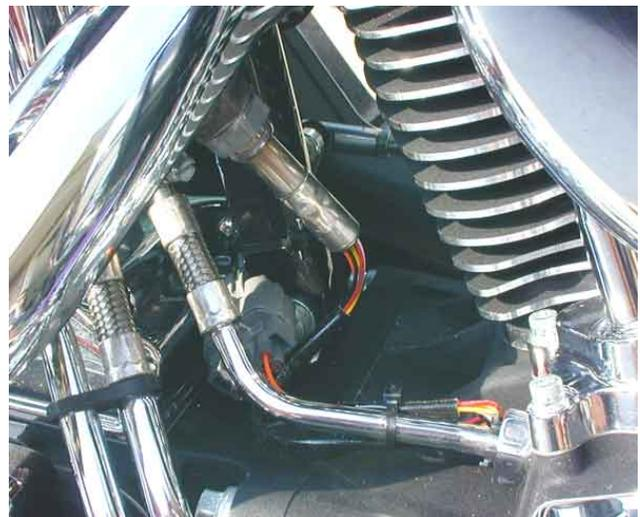
5. Install the WEGO unit. The WEGO is fully sealed for moisture protection. You can secure the WEGO with Velcro tape strips or a few tie wraps on the wire harness.
