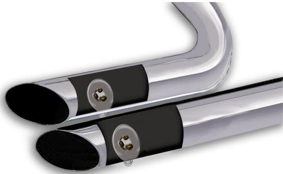
Use washers with an OD that is 2/3 to 3/4 the ID of the pipe (for example, 1-1/2" OD washers are suitable for pipes with an ID of 2" to 2.25"). Weld 1/4-20 socket head cap screws to the washers as shown. Drill holes at the bottom of the pipes about 2" from the end and use decorative acorn nuts to secure the washer assemblies. We suggest that you use stainless steel hardware.
